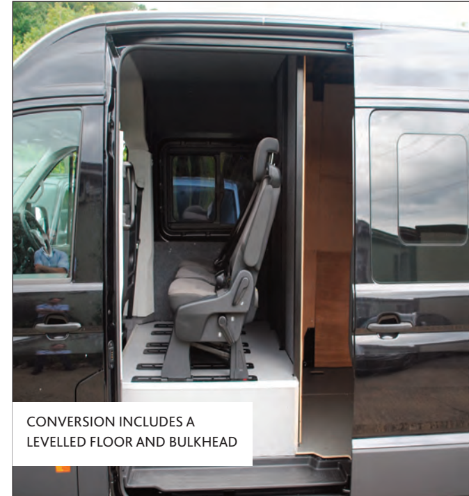
OEM SEATS FITTED TO CONVERT VEHICLE INTO A CREW VAN
