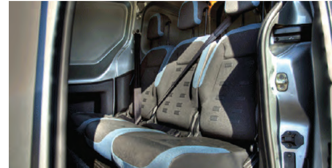
Installation of additional M1/M2 tested seats and seatbelts meeting all regulations and guidelines.
