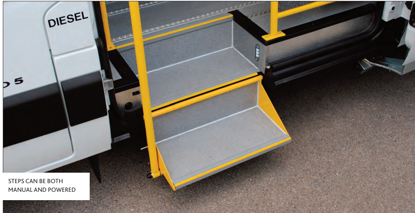
AUTOMATIC STEPS COMBINED WITH A POWERED DOOR
